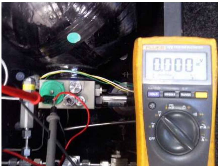
Figura 12. Electroválvula H2 (estado OFF).
